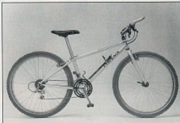
The radically sloping top tube on our smaller test bike created a good amount of standover height for our smaller test riders. Fairly standard angles with a longish fork trail create a more stable than aggressive bike for most trail riding situations.
